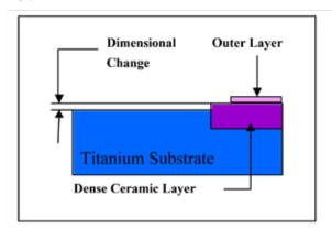
For some applications, buffing, tumbling or other means are used to remove the outer surface before the parts are put into service. Surface finishes as low as 16 Ra can be achieved with diamond lapping or honing techniques.
